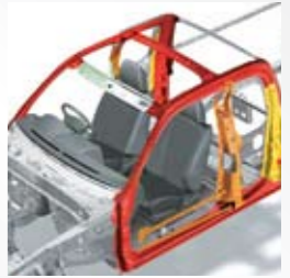
High strength Ranger's safety cell construction
