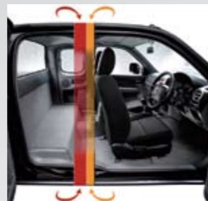
The Double B Pillar structure enhances protection in the event of a side collision*
