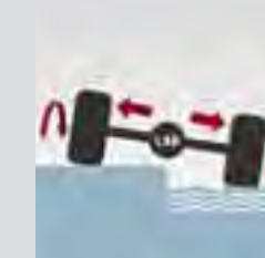
2-way Limited Slip Differential to power out of any low traction conditions
