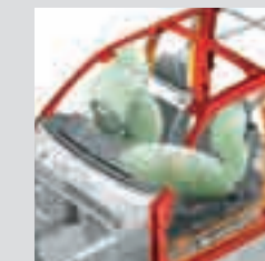
Large dual front airbags and high strength safety cage
