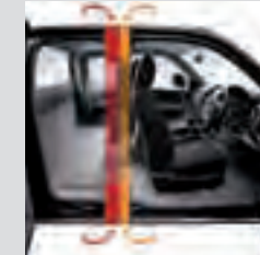
The Double B Pillar structure enhances protection in the event of a side collision
